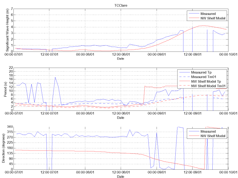
Figure A.2.12: Modelled and Measured Wave Conditions offshore Port Hedland (Beacon 15/16) - TC Clare.
