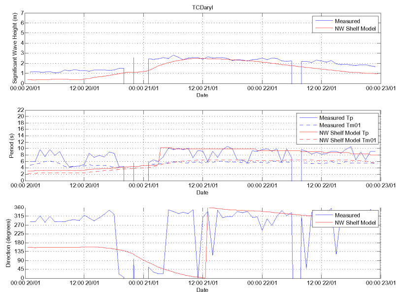
Figure A.2.13: Modelled and Measured Wave Conditions offshore Port Hedland (Beacon 15/16) - TC Daryl.
