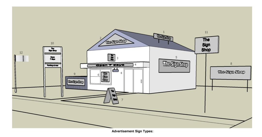
1. Above Roof 2. Created Roof 3. Projecting 4. Awning 5. Wall 6. Window 7. Ground Based 8. Hoarding 9. Fence 10. Monolith 11. Pylon 12. Tethered Note: The signs depicted in this diagram are those that can be diagrammatically illustrated. For all sign types allowed in the Town of Port Hedland, refer to the Definitions in Clause 4 and the corresponding Standards in Clauses 7 and 11.
