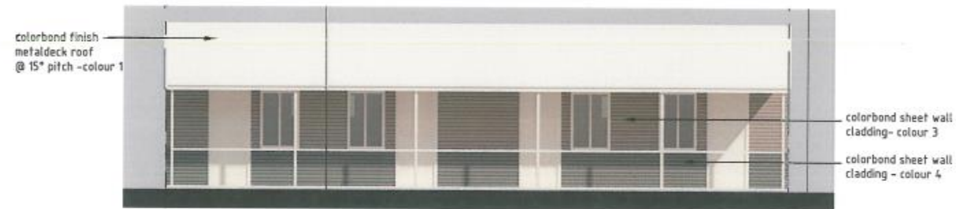
Accommodation Front Elevation
