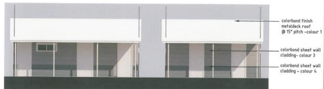
Ablution Block + Cleaners Front Elevation
