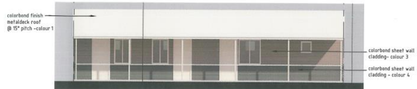
Accommodation Front Elevation
