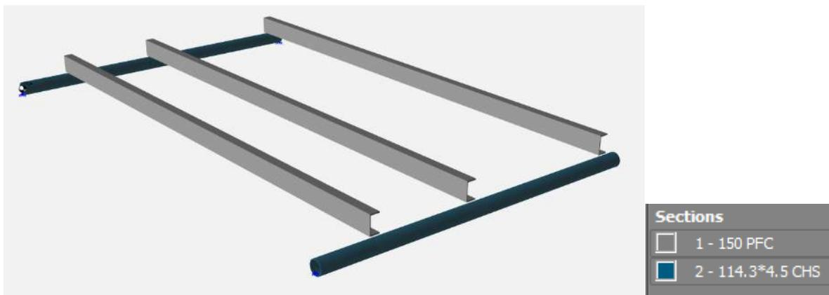
Figure 18: Space Gass model of typical platform
