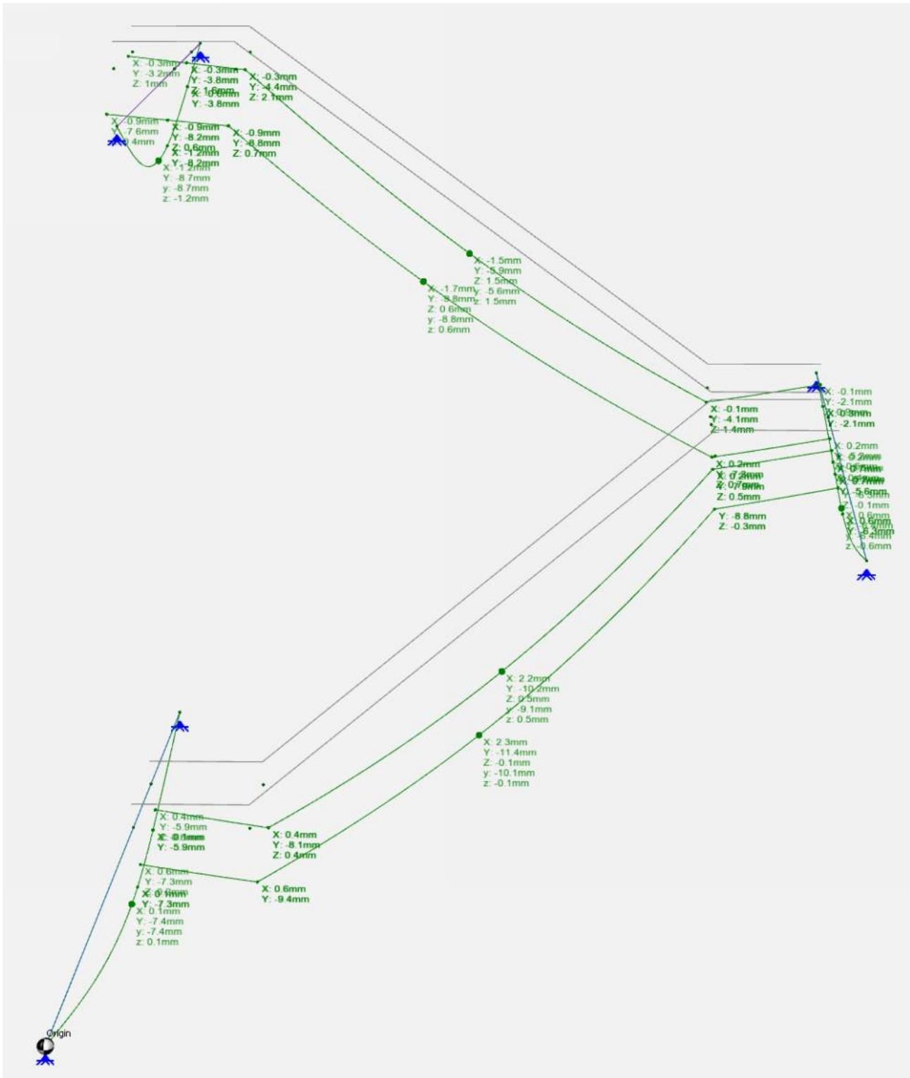
Figure 15: Deformation for Load Combination G+0.7Q
