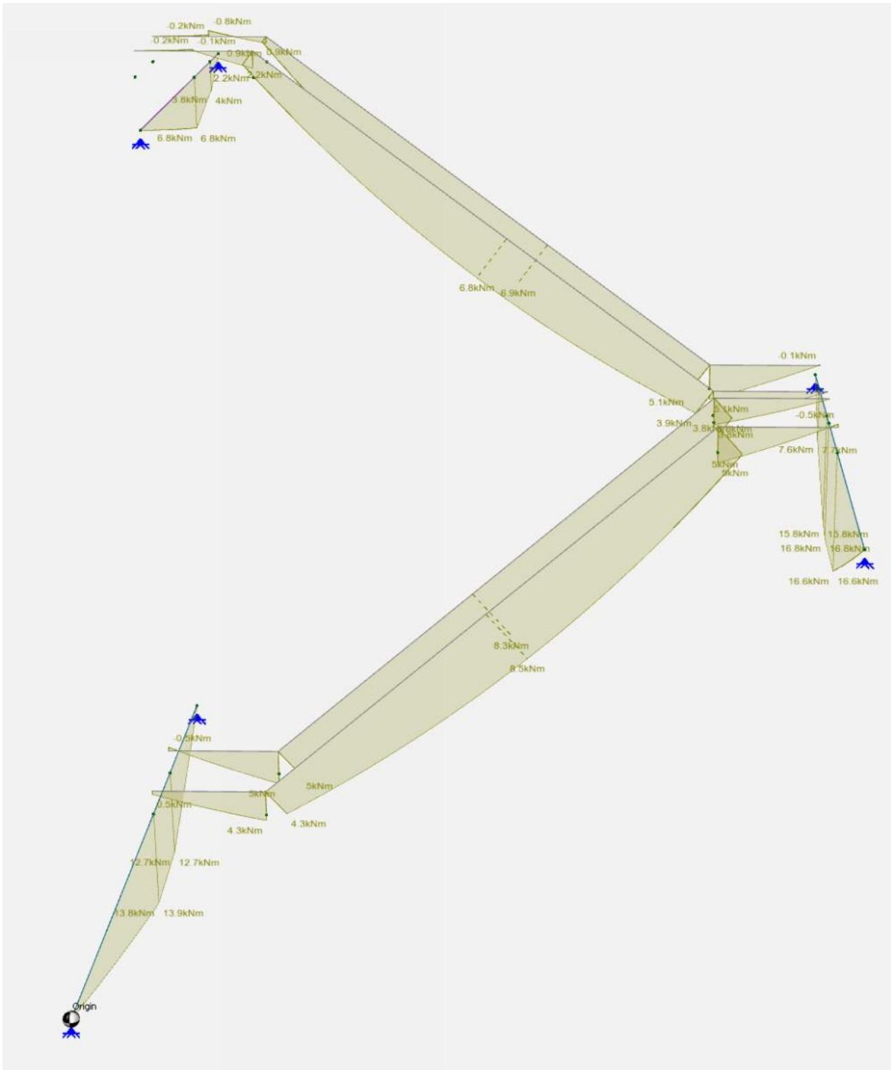
Figure 16: Bending Moment Diagram for Load Combination 1.2G + 1.5Q
