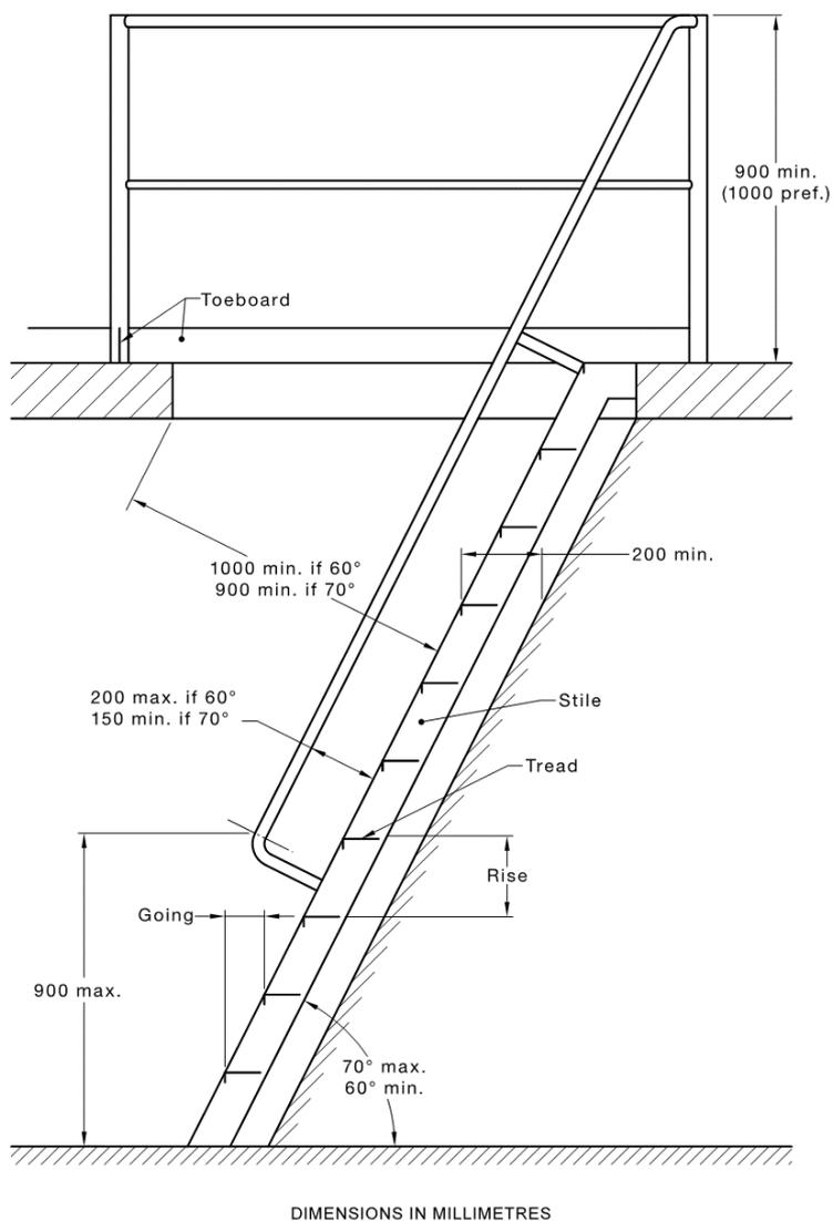
FIGURE 7.4 TYPICAL DIMENSIONS FOR STEP-TYPE LADDERS
