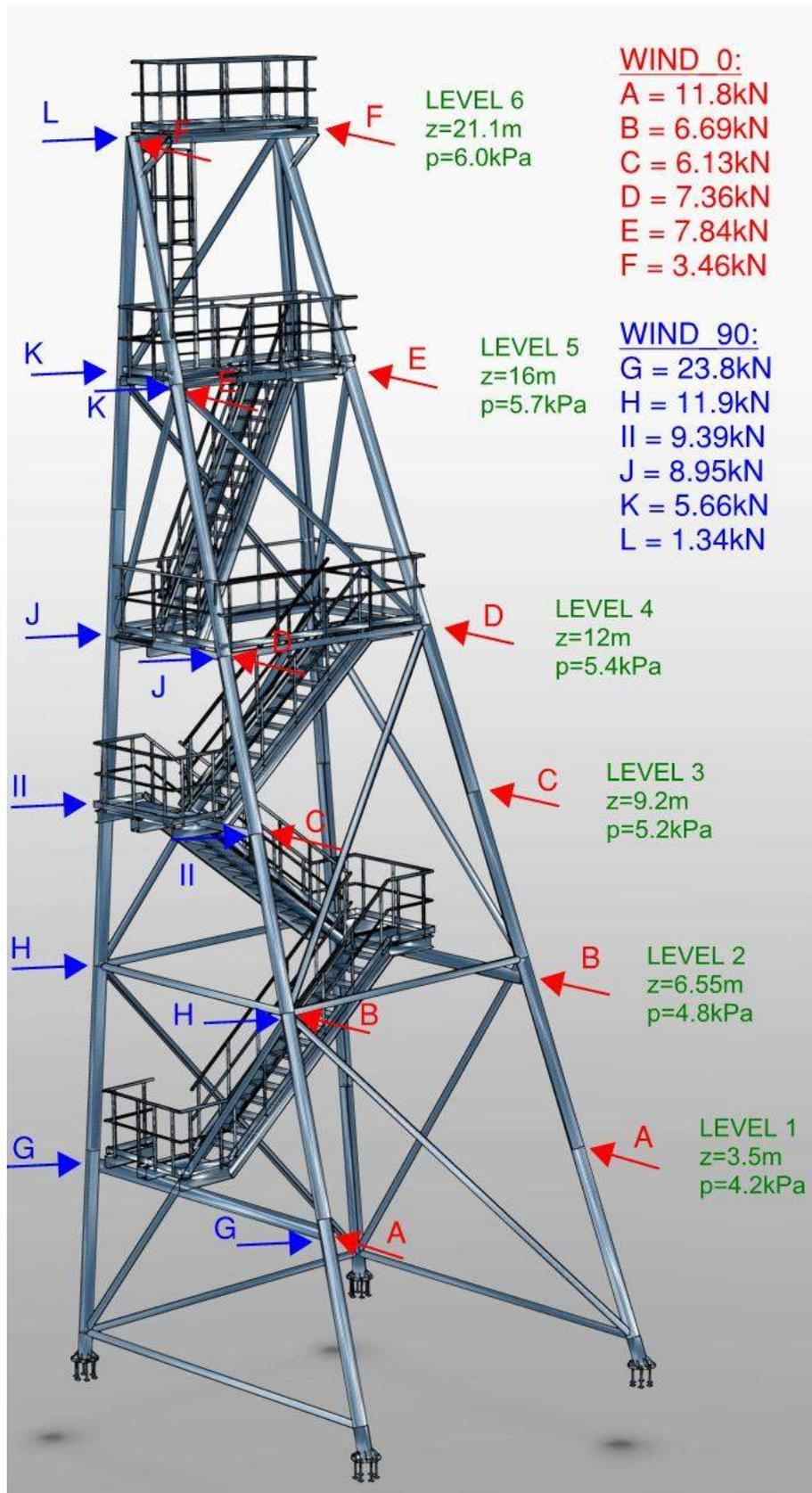
Figure 23: Wind Load Applied in SAP Computer Model
