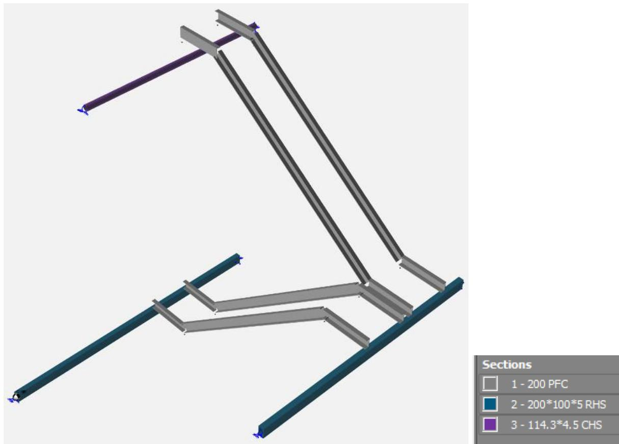
Figure 14: Space Gass model of stairway
