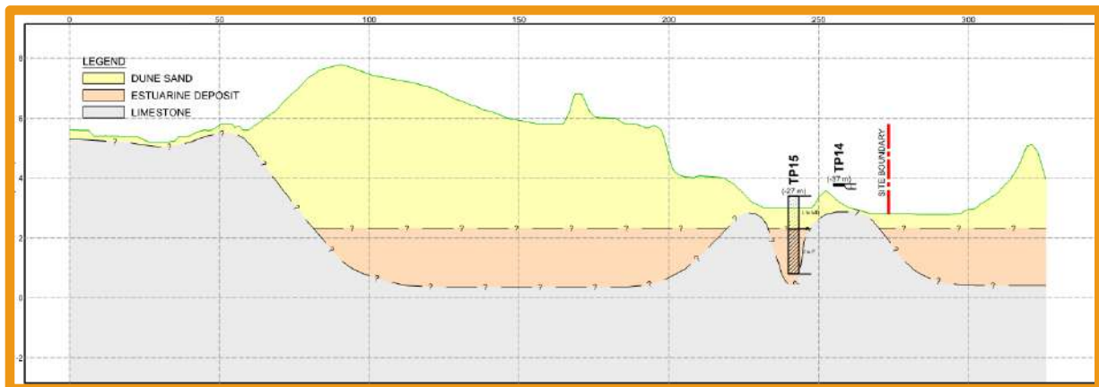
Figure 4-3 : Typical Geological Cross Section
