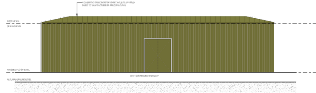
NEW LAUNDRY - FRONT ELEVATION
