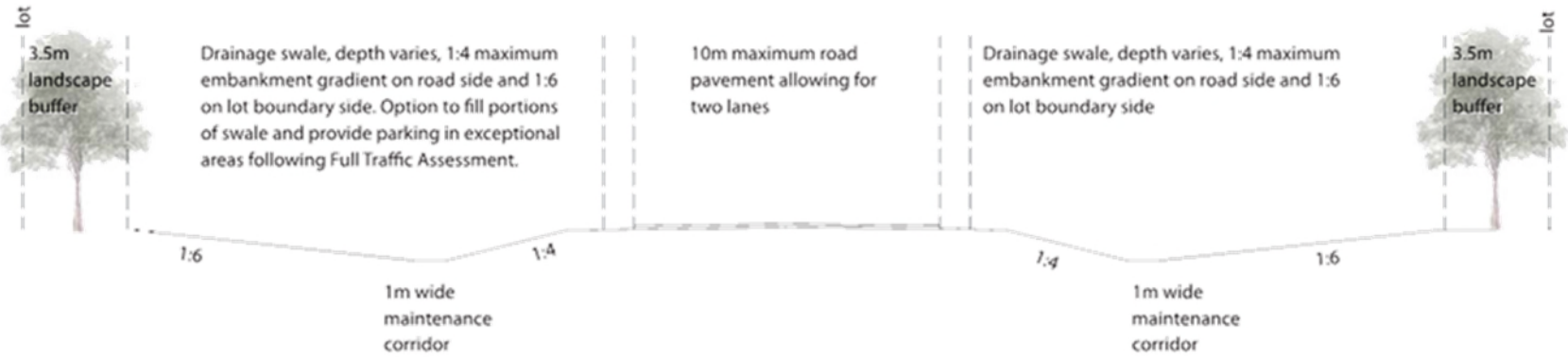
Section 2 - Local Distributor Road - 50m Road Corridor (typical) E.g Trig Street of Pinnacles Street.
