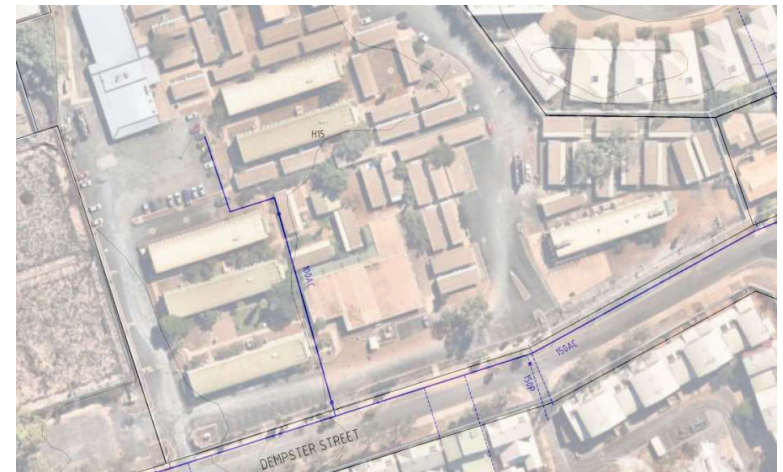
Figure 2: Illustration of Lot 2 being serviced with a 100mm water supply main.
