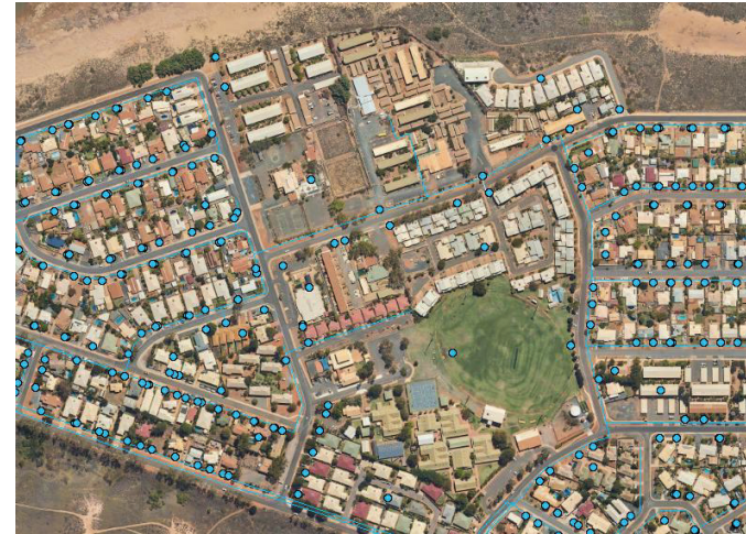
Plate 2: Reticulated water pipe (blue line) and water meters (blue dots) (SLIP 2025)
