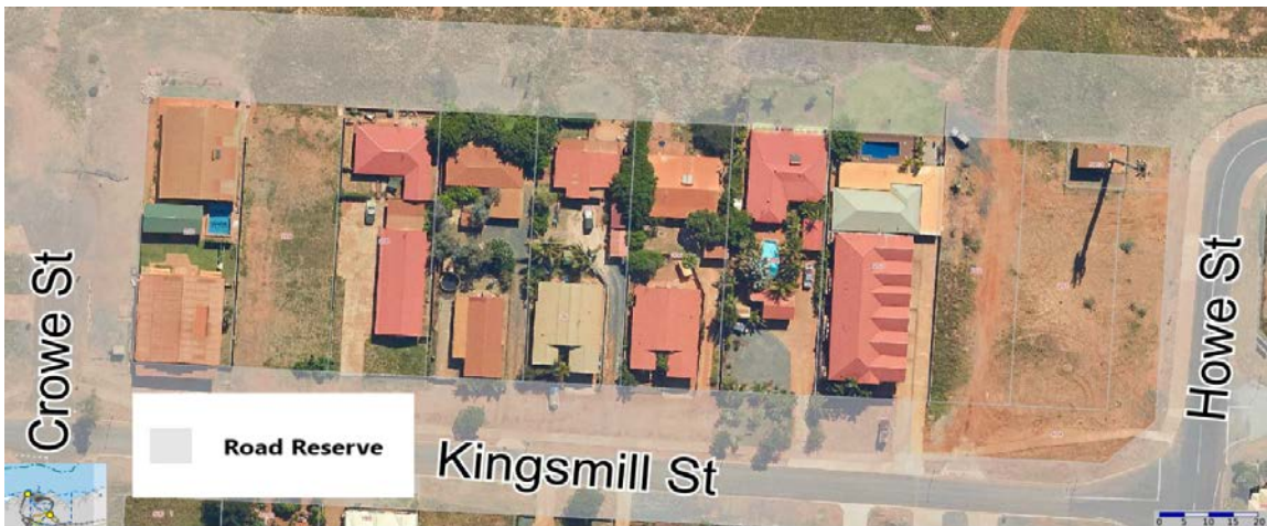
Fig 1 – Example of Kingsmill St Encroaching Property Boundaries
