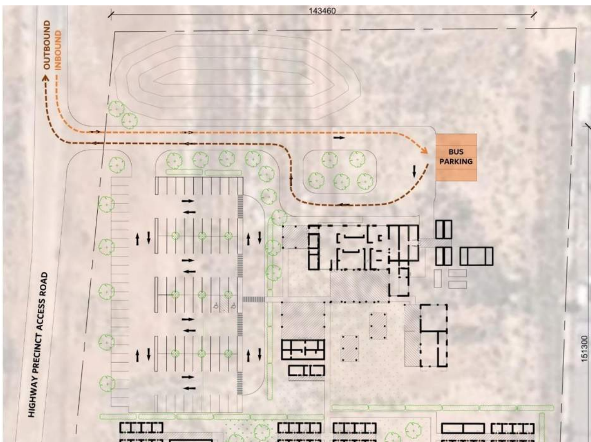
Figure 10 Proposed bus parking movements into and out from the site (base plan source: Grounded, 2022)
