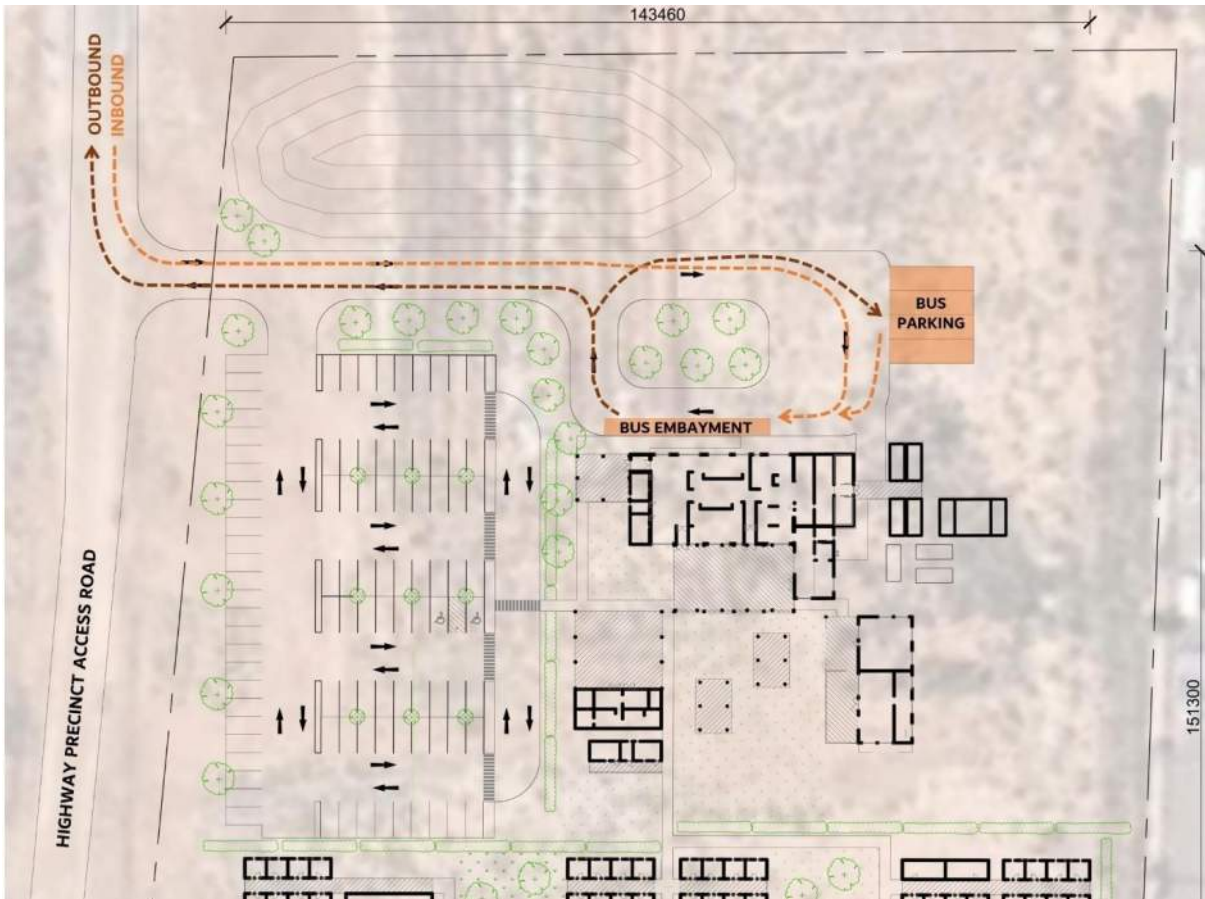
Figure 12 Proposed bus pick-up / drop-off and parking movements into the site (base plan source: Grounded, 2022)
