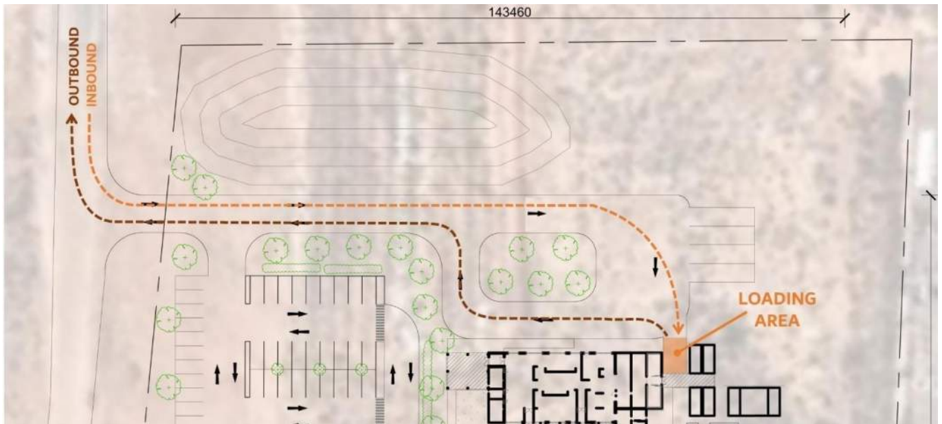
Figure 15 Proposed delivery and service vehicle movement into and out from the site (base plan source: Grounded, 2022)
